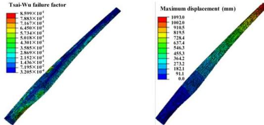
Fig. 5. Tsai-Wu failure factor and maximum displacement distribution of original laminating scheme of blade skins
