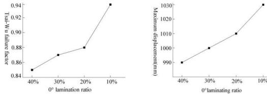
Fig. 3. Change curve of test index under different 0° lamination ratio
